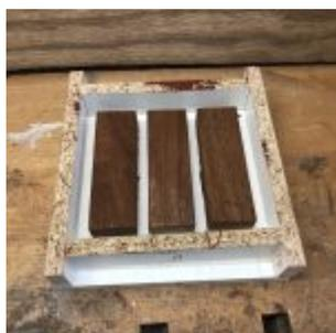
The negative mold for the Triple Double Silicone Mold
