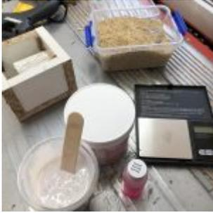
Mould, rice for obtaining volume, scales and silicone rubber.
