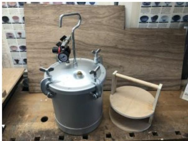
*Homemade vacuum chamber and caddy*
