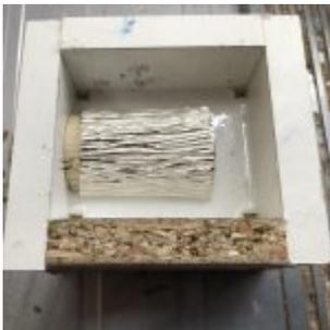
Partially filled mould with cured silicone showing register corner points.
